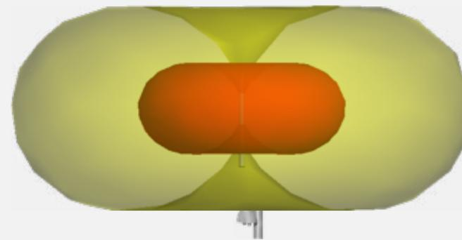
Typical multiband low gain omnidirectional antenna
